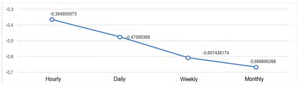
Fig. 65. Pearson's correlation coefficient for the series of electricity consumption and temperature data depending on the data averaging interval
